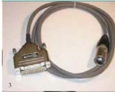
3. PC parallel-to-CAN cable. Required for PC comm using M800/880 ECU Manager software. Also used for firmware upgrades and logged data retrieval on the M800 family of ECUs running DOS EMP
