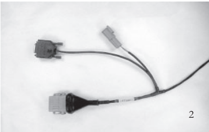
2. CIM cable, connects ECU, ADL, and PC to CIM. More rugged design for permanent installation in vehicles.
