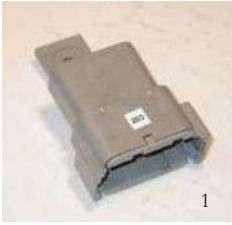
1. CIM module (computer-interface module) Converts TTL to RS-232 P/N: M CIM $164.00
